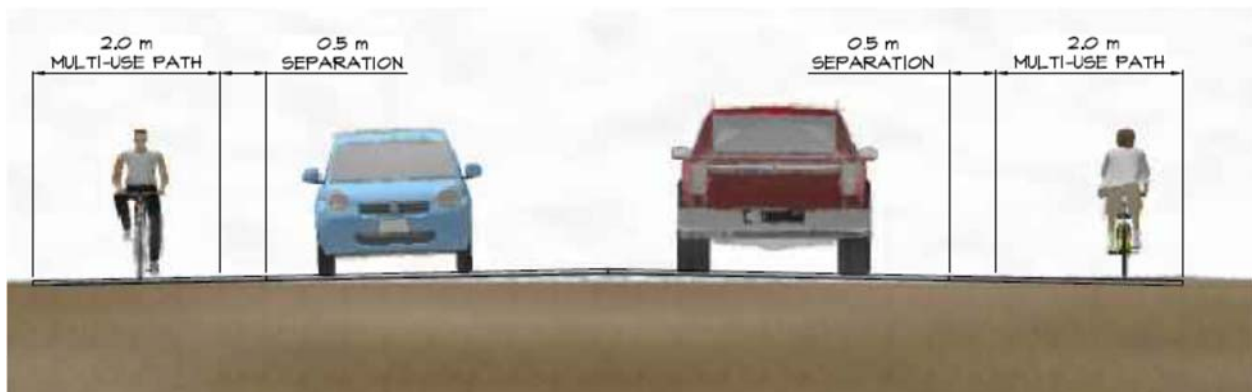
FIGURE 2 - EXAMPLE BUFFERED SHOULDER BIKEWAY CROSS-SECTION
